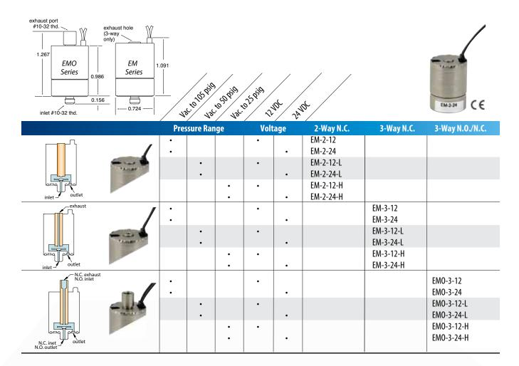
At just over 1" tall and less than 3/4" in diameter, the EM series is an ideal choice when space is critical. This reliable, proven design is housed in a miniature body with wire leads out the top to allow body rotation for close-center mounting. High flow combined with fast shifting speed, extremely high cycle life, and design flexibility make this valve a small wonder for demanding applications.
